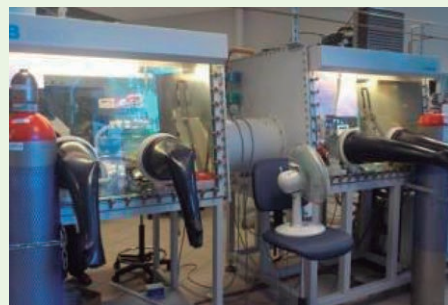
Glove box (under inert gas and positive pressure)
