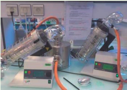
Drying device (heating under ~vacuum)
